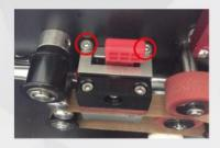
8.5 Remove the blade by lifting the rear of the blade then pulling upwards.
