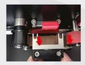
8.6 Install the replacement by sliding the front edge of the blade into the housing then firmly press down.
